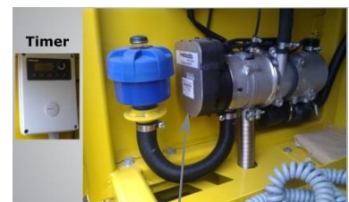
HEATING SYSTEM FOR ENGINE
