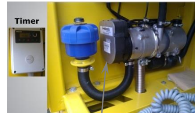
HEATING SYSTEM FOR ENGINE
