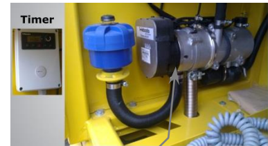
HEATING SYSTEM FOR ENGINE
