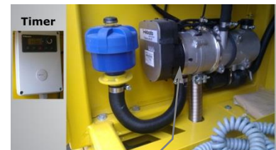
HEATING SYSTEM FOR ENGINE
