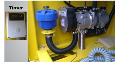
HEATING SYSTEM FOR ENGINE
