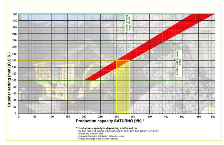
**EXAMPLE:** Feed material is granite (W<sub>i</sub>=16). If the crusher is set to a C.S.S. of 160 mm, the max. production will be between 300 and 340 t/h. Considering the bulk weight of the material of 1,6 t/m³ (see TECHNICAL INFO Page 3), the production capacity will be between 300 / 1,6 = 188 m³/h and 340 / 1,6 = 213 m³/h. For Granite (W<sub>i</sub>=16), the production will be in the middle range = approx. 320 t/h.
