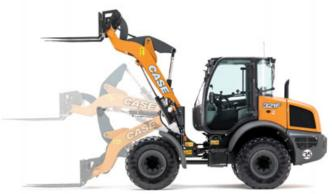
**Z-bar** is the most versatile linkage type. It offers more breakout force thanks to the 2 lifting cylinders and a higher dump height.
