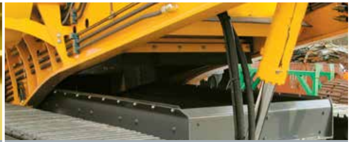
Patented hydraulic lifted chassis
