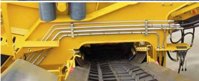
Steel hydraulic lines
